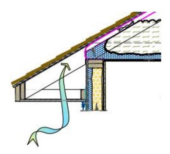
The soffit is any finishing material installed to cover the underside of a roof overhang. The soffit area usually runs most of the perimeter of the building but not always. Apart from aesthetic purposes like covering the exposed rafters making up the underside of your roof's overhang, soffits provide attic ventilation through perforations or vents in the material.
