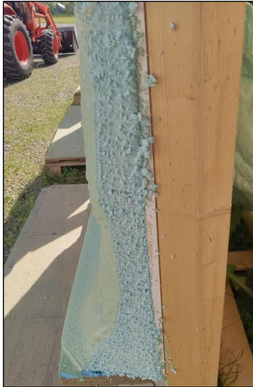
Figure 6. Day 1 SealTite One applied to test walls with sides trimmed
