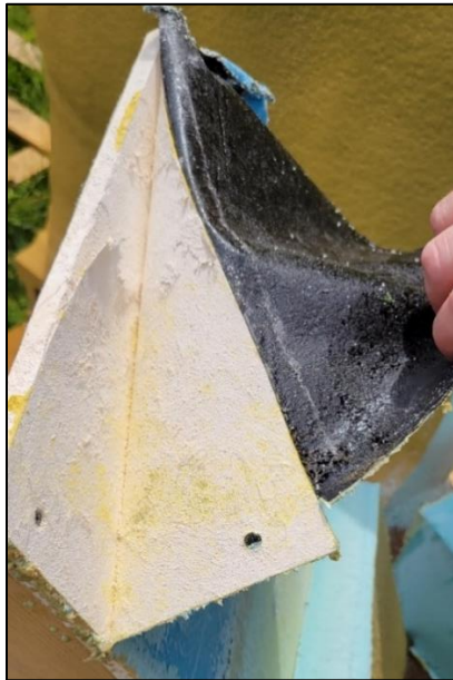
Figure 10. Attempts to pull Blueskin SA away from the gypsum substrate shows excellent adhesion. Adhesion failure occurred between the fibreglass facer to the gypsum.
