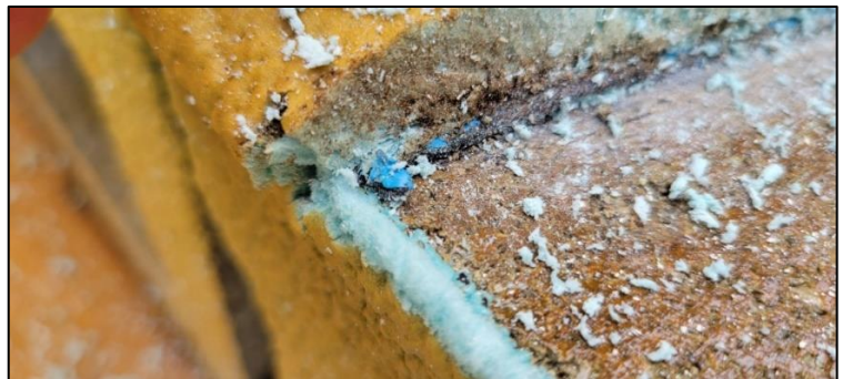
Figure 12. No cupping, curling, or warping after 3 weeks. SealTite One is flat. Blueskin SA is well adhered to CMU.
